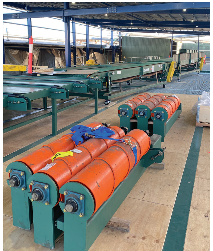
New spiral rolls for the drymill.
