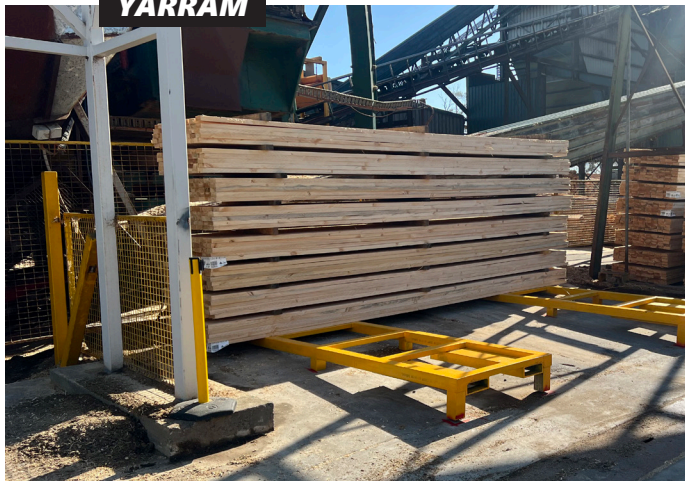
Pack Levellers were developed in Yarram for use of WIP piling stock for the slopped concret making the area safer.
