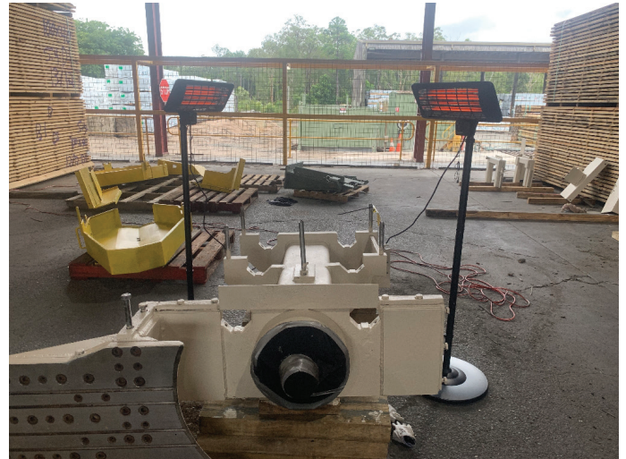
Quad LH Chipper Assembly twin Gas Heaters to cure the paint of the bearing quill assembly.
