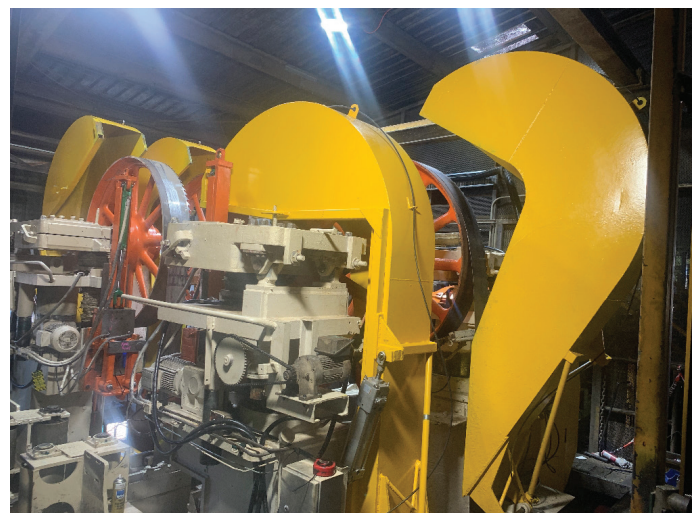
Quad LH Side Band Wheels re assembled ready for cutting logs.
